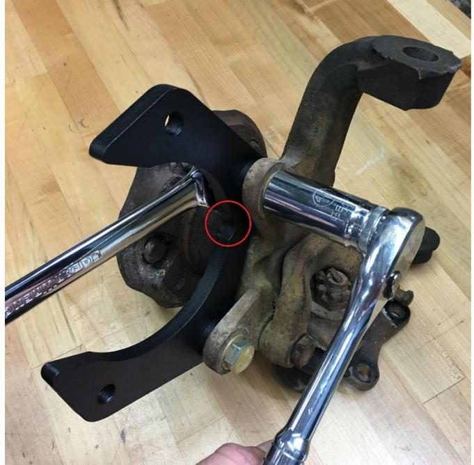
Reinstall the hub in the same way it was removed using the supplied cotter pin. You can now bolt on the caliper brackets using the included hardware and torque to **20 ft-lbs**. The caliper should be mounted to the back of the spindle. Make sure the **spacer** side is to the **INSIDE** and the **notch** for the caliper casting is **UP**.
