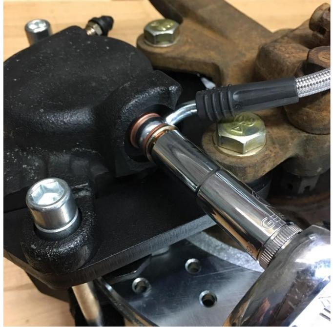
The calipers can now be installed using medium strength threadlocker (such as Loctite 243) on the threads of the two 7/16-20 caliper bolts and torque to **30 ft-lbs**. Then install the hose onto the caliper as shown. Be sure to install the crush washers on top and bottom of the banjo fitting.
