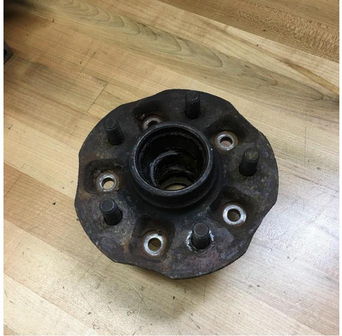
Remove the 5 bolts securing the rotor to the hub. The rotor can now be removed and discarded.
